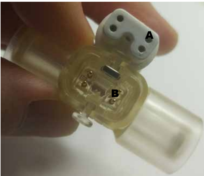
Figure 5: hot wire anemometer and connecting cable. A: Look for damage or discoloration (usually greenish) here as it may affect signal quality. Look for corrosion at the base of the connecting pins. B: The cable should connect such that it is at the top of the sensor.
