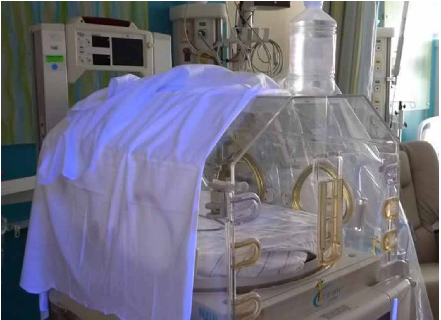
Figure 5: When curtains were retracted, the fabric on the exterior of this incubator did fluoresce, but the interior did not; this suggests that the incubator transparent cover did not transmit UV-A.
